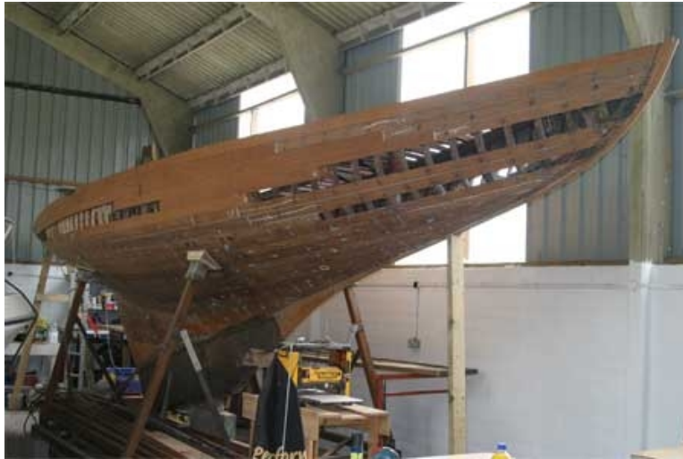
Under going the restoration below the waterline completed and topsides commenced
